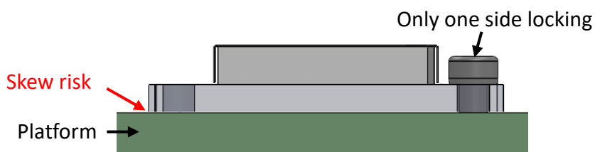
Figure 4.1.1.2.11 Avoid skewing after tightening the unilateral screws
