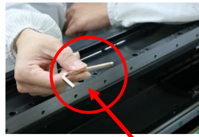
Figure 4.1.1.3.2 Use non-magnetic tool to install the stator
