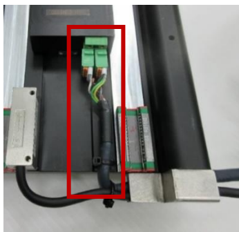
Figure 3.3.1.4.16 Fix the motor cable by cable tie and cable tray
